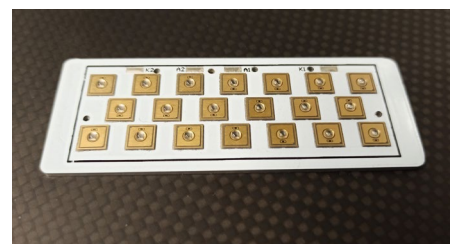
Illustration 3 2.1 Watt UVC-LED module 265 nm (Fraunhofer IOSB-AST)
